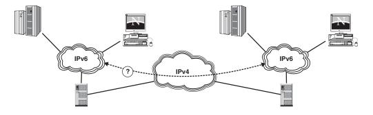
Figure 10. Communicating between IPv6 islands in an IPv4 world
