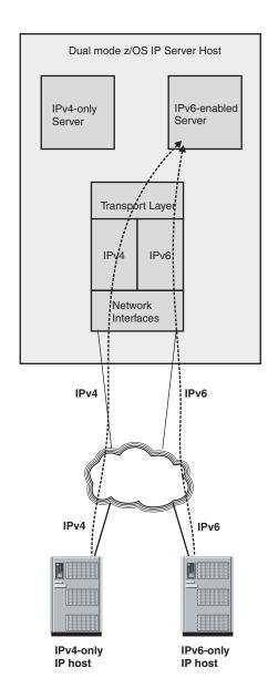
Figure 12. IPv6 application on dual-mode stack
