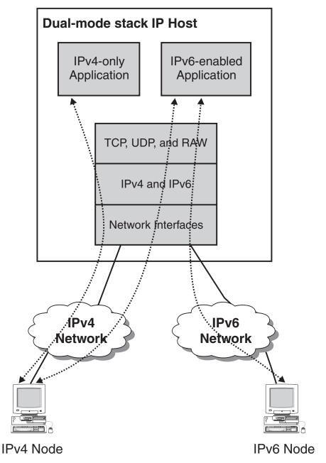
Figure 21. Dual-mode stack IP host
