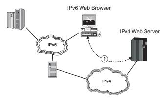
Figure 11. Communicating between IPv4 and IPv6 applications
